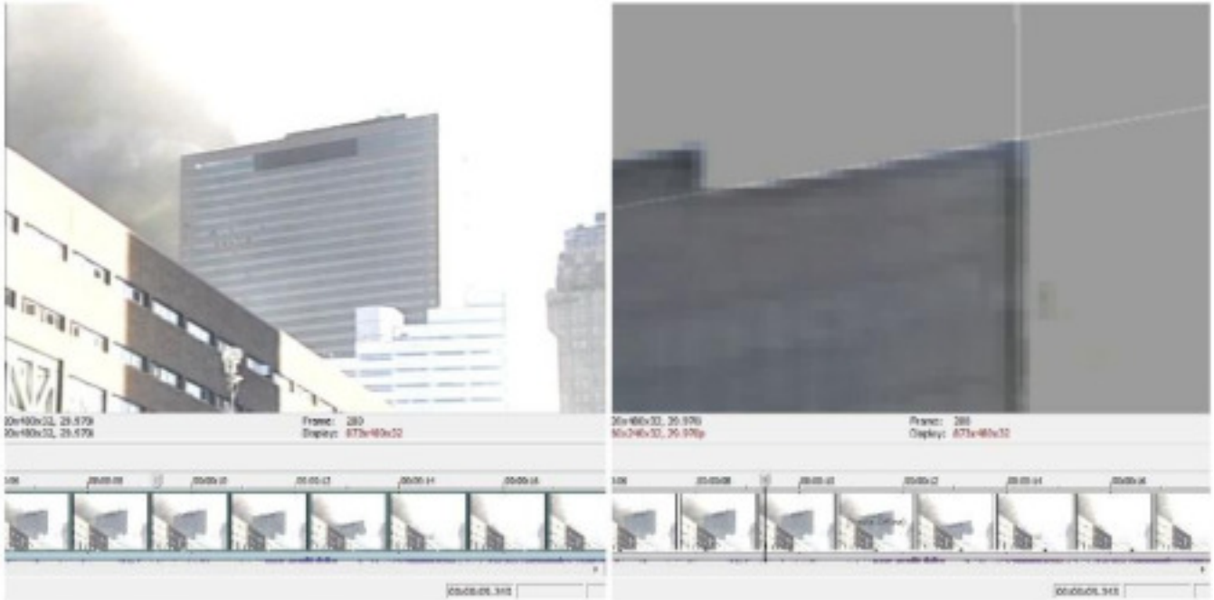
Figure 16 – At frame 280 (9.343 s, NIST's "0.0 s"), there is still slight displacement eastward as the northwest corner is oscillating back to its baseline position.
